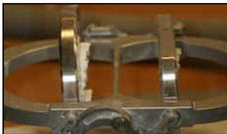
**Fig. H** The Eco milling machine can be set to different angles to mill every corner of the restoration.
